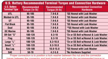
(never between the connector and lead terminal) and apply the recommended torque or enough torque to completely compress the lock washer without deforming the lead terminal
